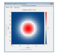
Data arrays normally include complex fields (or alternatively double arrays) as data and have additionally coordinates and sampling information specified. Hence, they can be visualized as fields. Data arrays can have multiple subsets, which all need to have the same sampling parameter (normally used for the components of a field).
