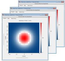
A set of data arrays contains multiple individual data arrays as subsets. Different to the case of the data array, these subsets can all have different sampling parameter. Normally these subsets represent the wavelength modes of a field, but could also be used for anything.
