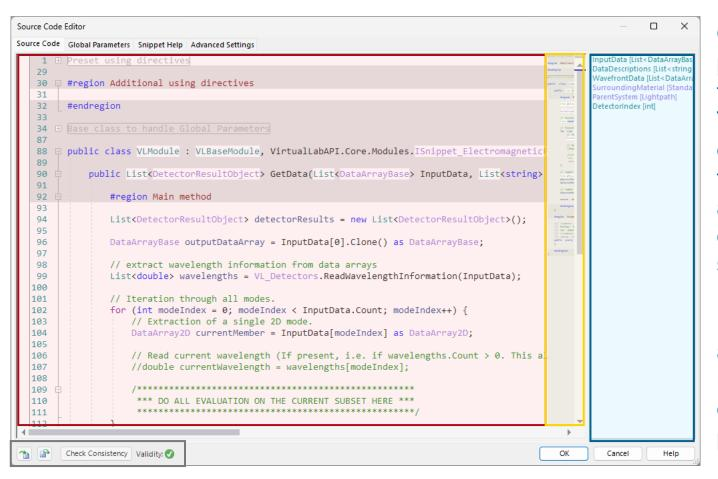
On the right side all global parameters are listed with the respective classes. This includes parameters defined by the user (see following pages) as well as pre-defined parameters depending on where the snippet is found. For Detector Add-ons the input field (with wavefront) and the surrounding material are e.g. predefined global parameters.
