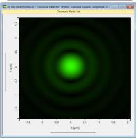
A Chromatic Field Set is a special version of Set of Data Array in which the subsets do need to represent the wavelength modes of the field. It offers additional functionalities and views in the main window.
