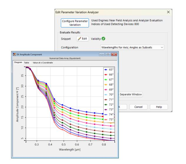
This tutorial demonstrates the use of the Parameter Variation Analyzer to calculate important properties from ellipsometric analyses. Its flexibility allows the automatic calculation of results based on variations in wavelength, angle or both. The user can thus be provided with 1D plots representing phase differences and amplitude components over angles of incidence and/or wavelengths.
