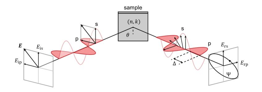
Ellipsometry measures the reflection for the s- and pcomponent, which can be described as complex reflection (or Rayleigh in case of a grating) coefficients ( $R_p$ ,  $R_s$ ):
