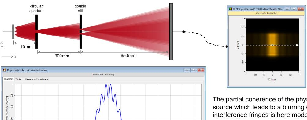
The partial coherence of the physical extended source which leads to a blurring of the interference fringes is here modeled with the set of self-correlated but mutually incoherent point sources presented in the previous slide. The interference patterns of each of the point sources do not coincide, causing the characteristic loss of contrast.
