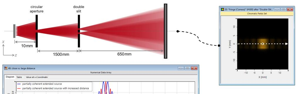
By increasing the propagation distance in front of the double slit to 1500mm, we demonstrate the predictions of the van Cittert-Zernike theorem, in that the light generated from two incoherent sources will appear coherent from far away. This is evidenced by the increase in contrast that occurs for a larger distance in front of the double slit.
