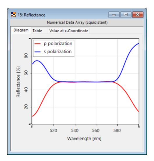
The reflectance diagram indicates that the non-polarizing beamsplitter cube splits the incident beam independently of polarization within the operating wavelength range of approximately 525 nm to 575 nm.
