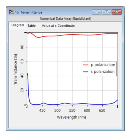
In contrast, the polarizing beam splitter cube only transmits the p-polarized component of the incident light within its operational wavelength range (approximately 420 nm to 650 nm).
