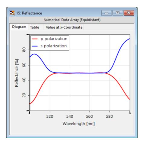
This use case presents the simulation of optical beam splitters, including both polarizing and nonpolarizing types, using VirtualLab Fusion software. An appropriate layer configuration is imported, followed by a wavelength scan to evaluate the performance of the beam splitters.
